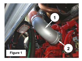
2. Please replace the OE elbow by the reinforced version referring to the step-by-step instructions further in this Bulletin.
