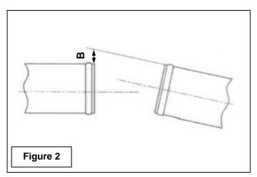
In order to avoid chafing of the silicone liner, the pipe ends should not butt the reinforcing rings. A minimum clearance of 1/8" is required (Figure 3).
