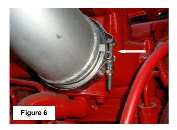
5) Slacken the lower flex hose CT clamp and detach and discard the elbow. Reclaim CT clamps 10617357, V-band clamp 11085406 and O-ring 11106808 if they are serviceable.
