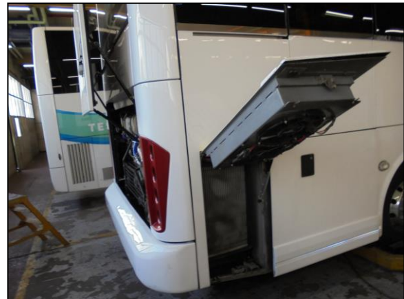
Figure 2: Access door with electric cooling fans for charge-air cooler (at the RHS of the vehicle) (CX45)
