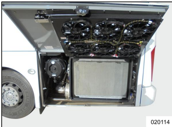
Figure 1: Access door with electric cooling fans for radiator (at the LHS of the vehicle) (CX45)
