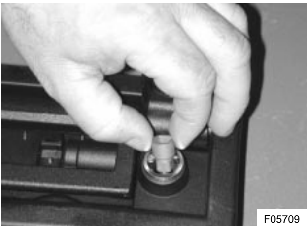
Figure 8: Cam drive installation
