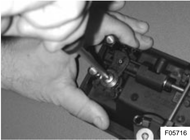
Figure 15: Securing the cam drive screw
