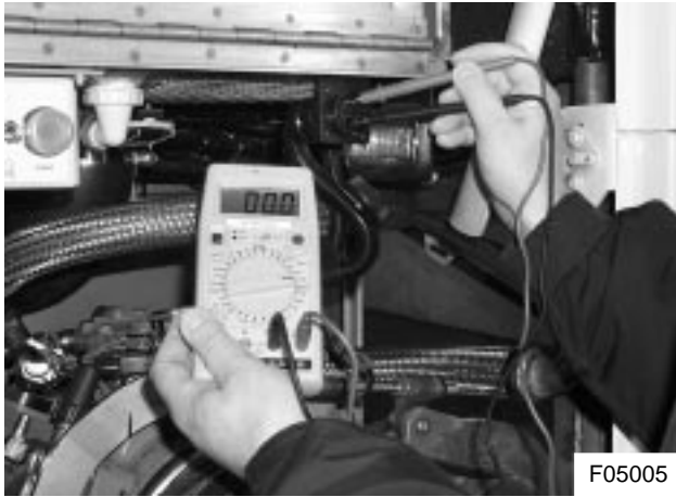
Figure 4: Testing with a multimeter
