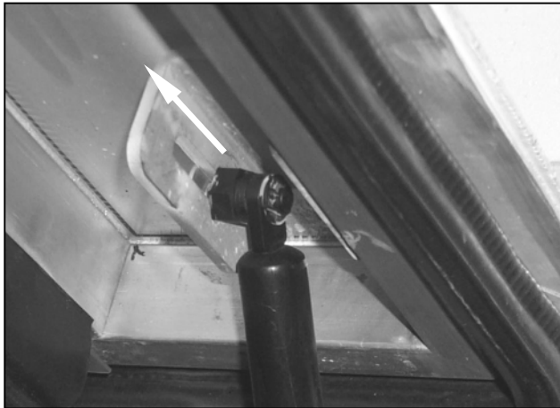
Figure 8: Upward pivot movement in door bracket slot
