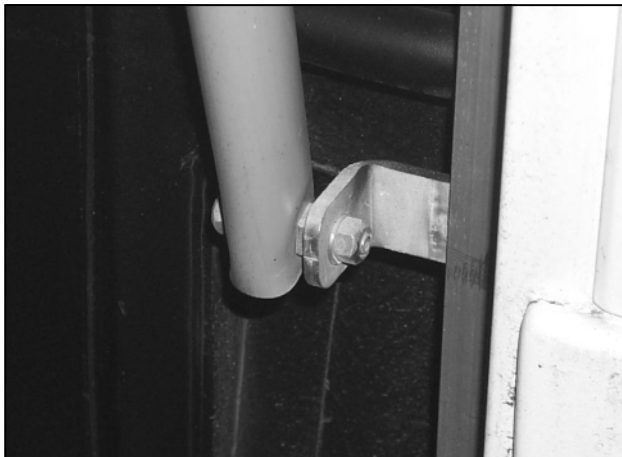
Figure 9: Gas spring to chassis pivot and fasteners
