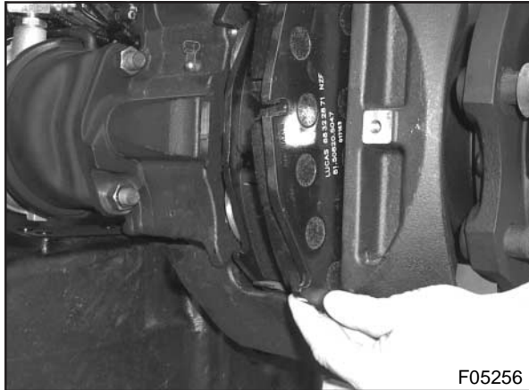
Figure 34 Brake pad removal
