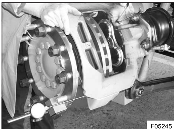
Figure 10 : Tilting the caliper
