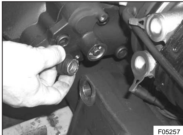
Figure 32 : Adjuster stem cap removal
