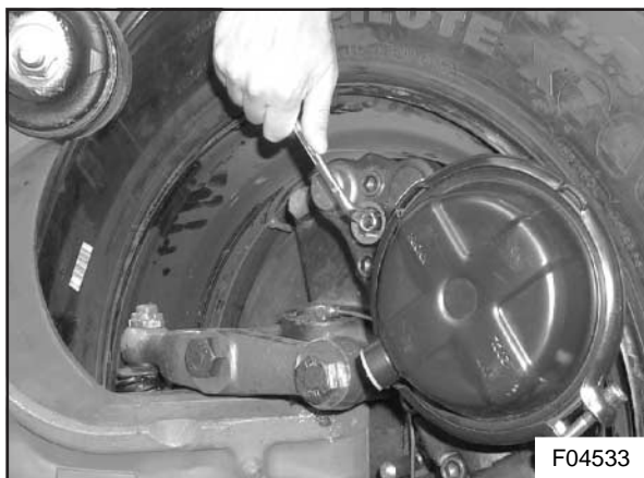
Figure 18 : De-adjusting the brake pads
