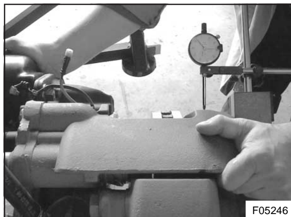
Figure 12 : Tilting the caliper
