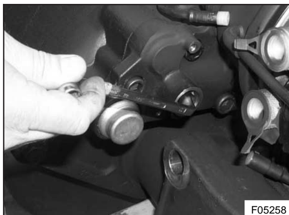
Figure 33 : De-adjusting the brake pads
