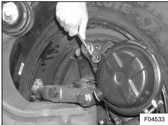
Figure 7 : To turn the adjuster stem with a box wrench
