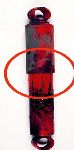
Shock is Leaking
