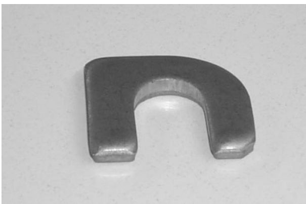
Figure 1: Stamped 5 mm carbon steel shims show unequal thickness and are no longer recommended for accurate suspension alignment purposes
