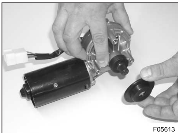
Figure 8: Wiper motor dust cap installation (for the sake of clarity shown with the motor out of the coach)
