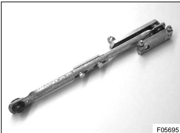
Figure 12: Bell crank and clamp assembled with left-hand tie bar
