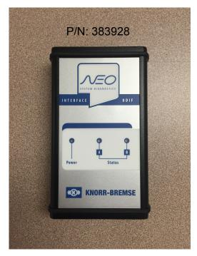
Van Hool specific adapter. This device will allow connection between the coach DMUX diagnostic port and the Knorr-Bremse UDIF.
