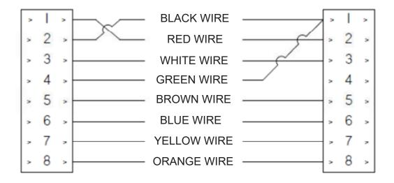
Moving forward, a plug and play adapter harness will be provided with a new mirror purchase. When replacing the mirror simply install the harness shown below to avoid wiring modifications. The adapter harness is not available separately.
